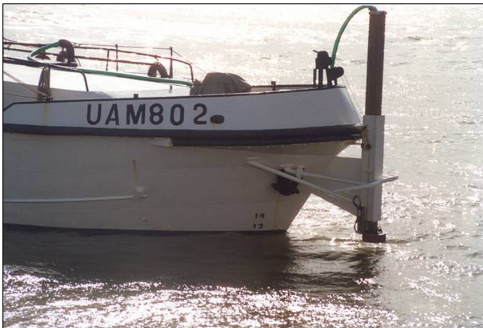
Fig. 3.19 "Transducer installation over the bow"
