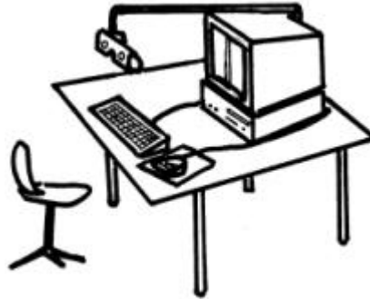
Fig. 6.51 "Digital stereo-plotter scheme"
